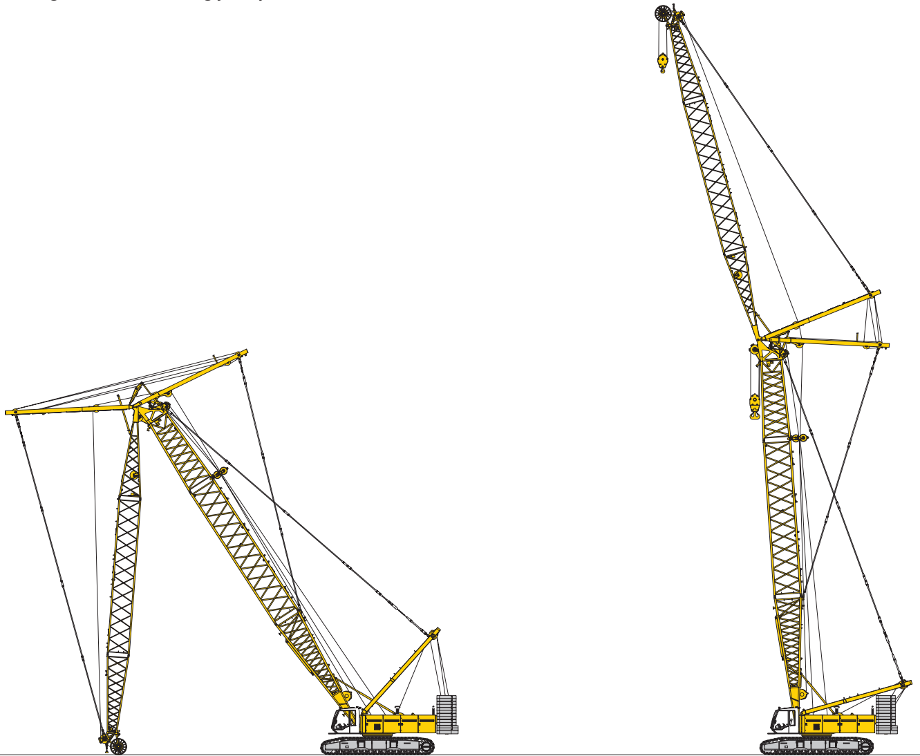
Erecting of main boom and luffing jib
