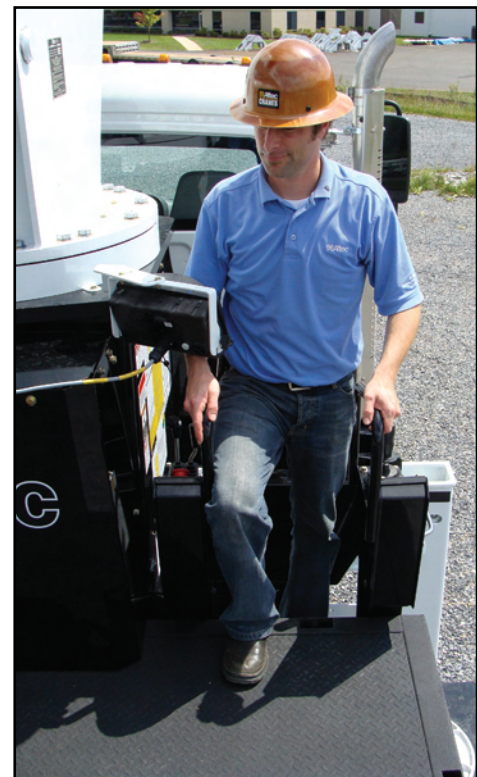
Walk Through Control Stations
