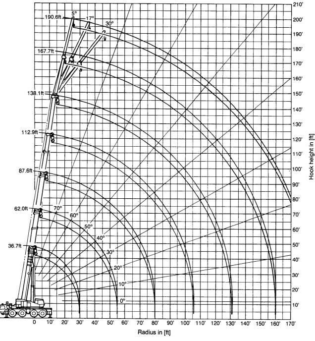
NOTE: Operating Radius is measured in feet from Axis of Rotation. Boom and jib geometry shown are for unloaded condition and machine standing level on firm supporting surface. Boom deflection and subsequent radius and boom angle change must be accounted for when applying load to hook.
