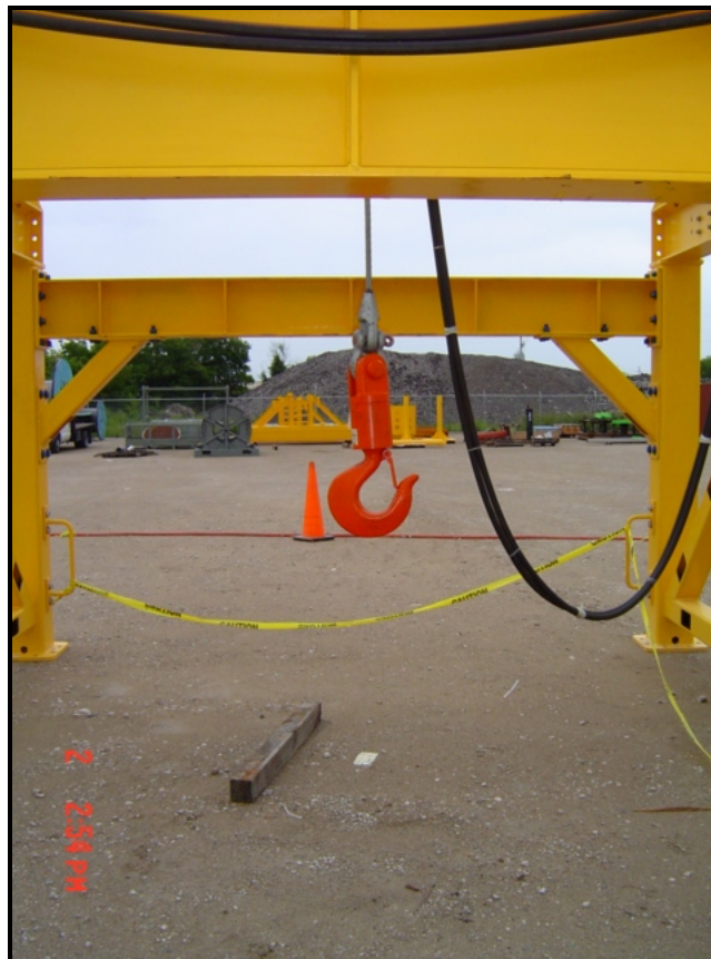
Figure 13 - Wire End Termination and Swivel Hook
