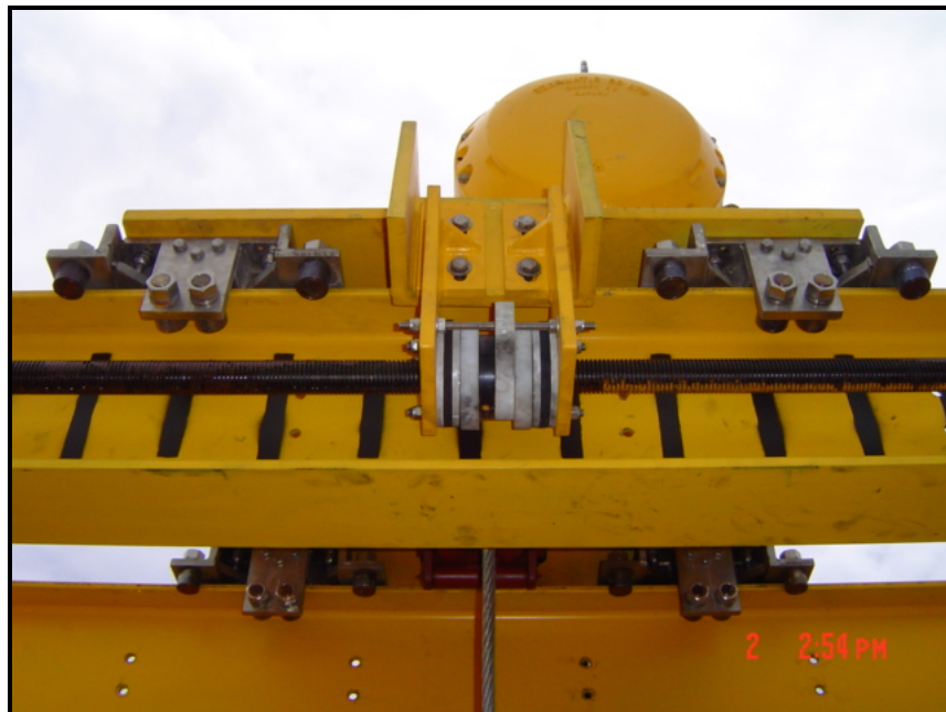
Figure 8 - Stainless Steel Rollers and Acme Drives
