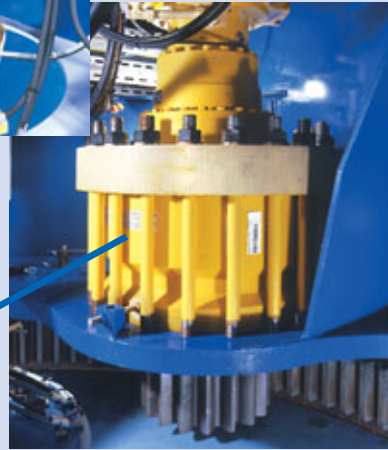
Modular designed slewing gear drive unit
