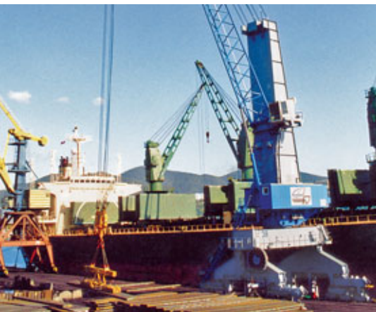
Gottwald Harbour Cranes can be supplied not only on a tyre-mounted chassis but also on a rail-mounted portal or barge. Seen here as an HSK 170 EG Portal Harbour Crane handling steel in the Port of Tuapse, Russia.
