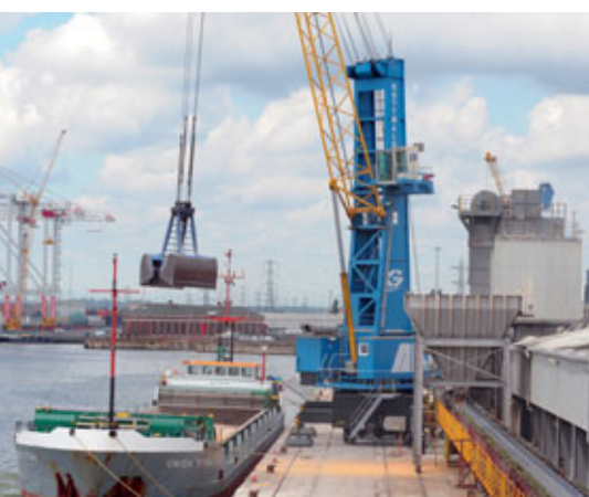
HMK 170 EG handling bulk material, such as scrap and agribulk, at the Port of Southampton, United Kingdom
