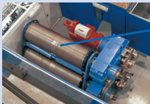
Two hoists for 4-rope HMK 170 EG
