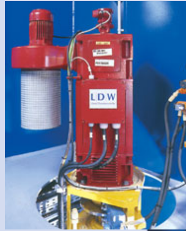
Modular designed slewing gear drive unit
