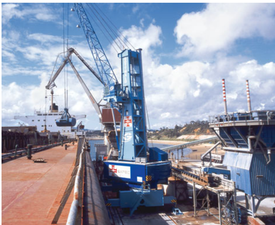
HMK 170 EG handling fertilizer at Sapec, Portugal: the field-tested H-shaped stabiliser arrangement enables the crane to operate even in areas with a minimum of working space
