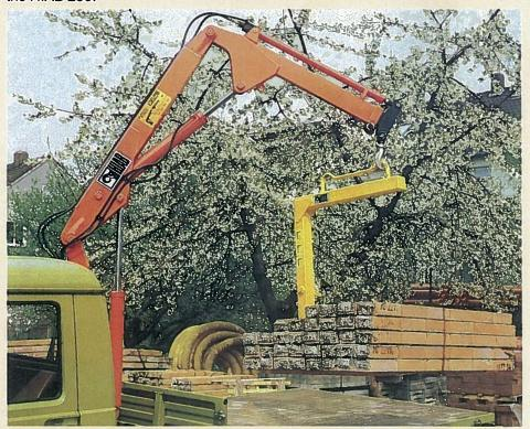
In the AU version the HIAB 250 can also be mounted at the back end of the truck bed.
