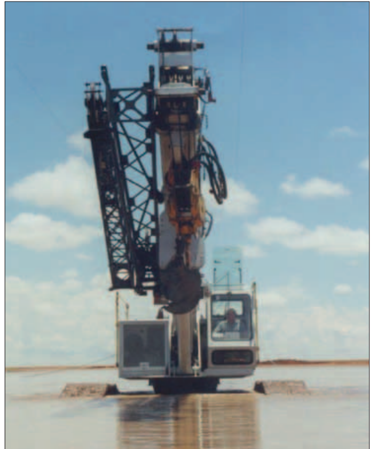
■ Low ground bearing pressure, fully sealed track drives and bearings, and high ground clearance allow the Mantis crane to traverse through extreme conditions. Above picture shows optional complete auger kit.
