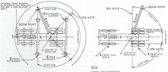
THESE LINES DETERMINE ANY LIMITING POSITION OF ANY LOAD FOR OPERATION WITHIN WORKING AREAS INDICATED
