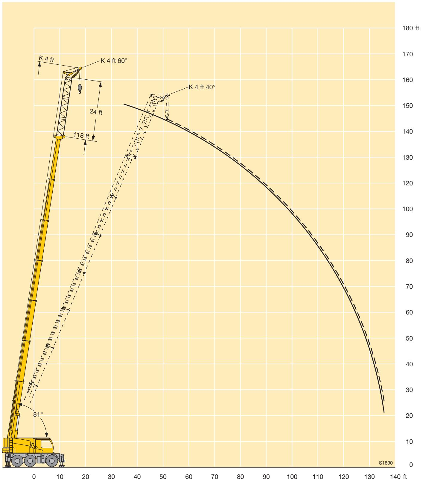
**Lifting capacities on the hydraulically variable folding jib with boom extension**
