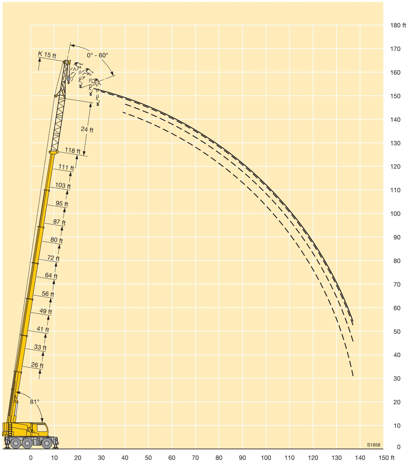
**Lifting capacities on the hydraulically variable folding jib with boom extension**
