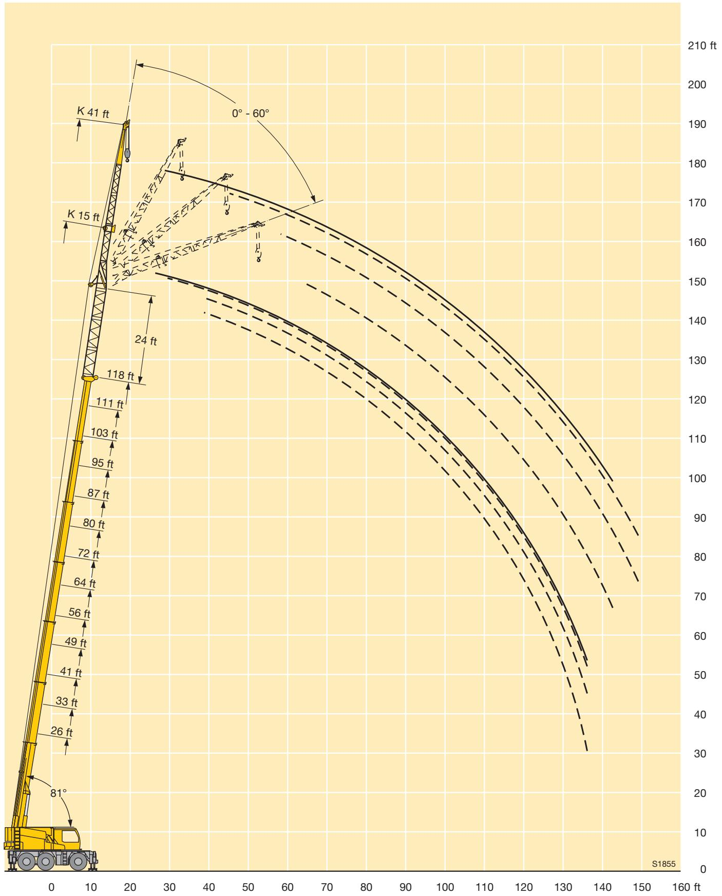
**Lifting capacities on the hydraulically variable folding jib with boom extension**
