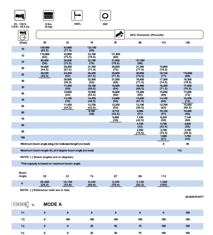
Regardless of counterweight and outrigger spread configuration, no deduct is required from the main boom charts for a stowed boom extension. However, the LMI system still monitors the effect of the stowed boom extension and will display a load value which will vary with changes in boom length and boom angle. To achieve maximum boom capacities, the boom extension must be removed from this crane.
