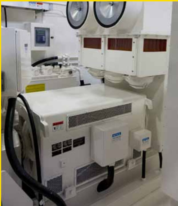
A reliable P&H AC Main Motor is housed within the 320XPC's spacious machinery house.
