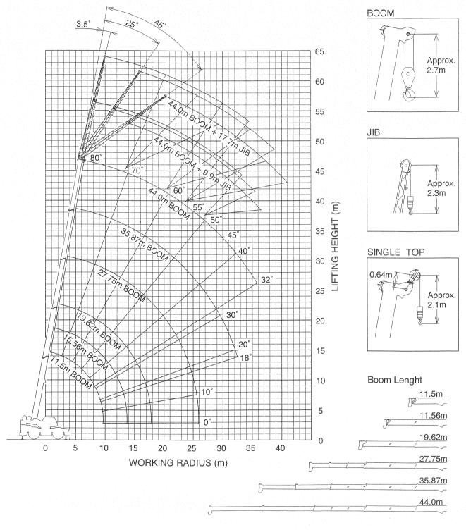
**NOTE:** The above lifting height and boom angle are based on a straight (unladen) boom, and allowance should be made for boom deflection obtained under laden conditions. The above working range is shown on condition with outriggers fully (7.2m) extended.
