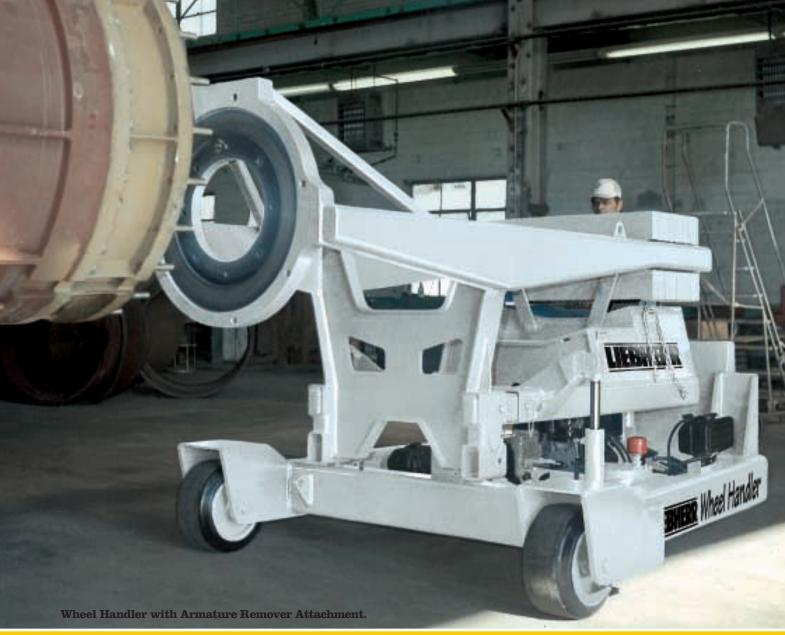
The Wheel Handler has been designed to aid in the installation and or removal of wheel motors used on diesel electric haulage equipment. The range of motion, including lift, skew, propel and steering by the use of joystick controls of this self propelled maintenance tool allows installation or removal of wheel motors or other large components to be significantly shortened.
