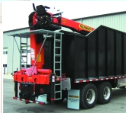
The crane can also be mounted at the rear of the truck for added flexibility.
