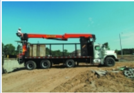
The inline boom stores between the cages
